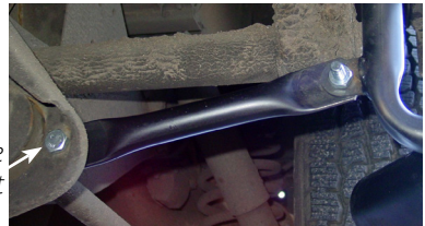
Rear brace arrangement passenger side looking back
